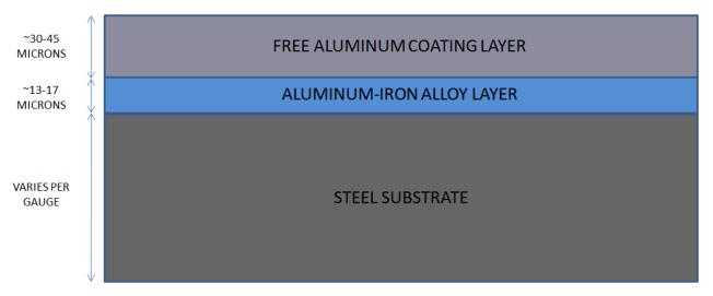
The gauges used in this study measured the overall thickness of the steel pipe as well as the free aluminum coating layer. The aluminum-iron alloy layer was not directly measured, but was estimated using the known thicknesses of these layers from decades of metallographic analysis.
