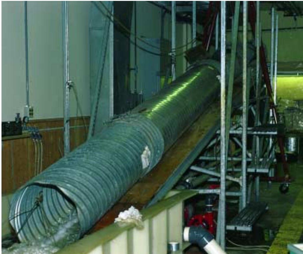
FIGURE 1A. Accelerated Abrasion Test Apparatus.
