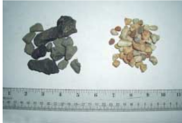
FIGURE 2. Bedload Materials ( \frac{3}{4} " trap rock on left, \frac{3}{8} " local stone on right)
