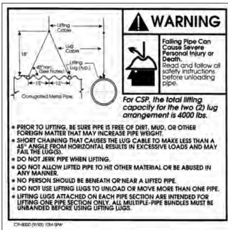
■ Figure 10.12a Lifting lugs for pipes to 4000 lb.
