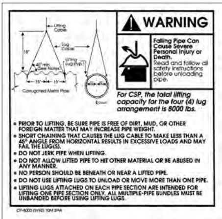
■ Figure 10.12b Lifting lugs for pipes to 8000 lb.
