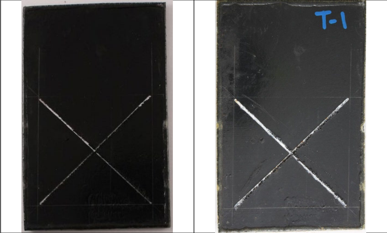
ASTM A742 Polymer laminate over Galvanizing
