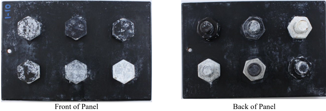
Figure 20: Example Panel After 60 Cycles
