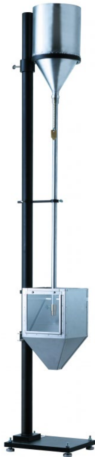
Figure 2: ASTM D986 Testing Apparatus
